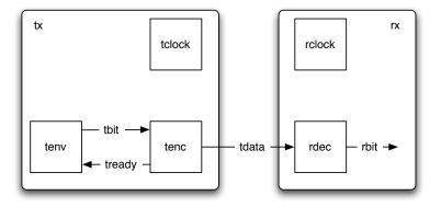
Just the encoder (tenc), decoder (rdec), and constraints are protocol-specific.
