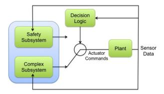
Figure 9: Simplex architecture (reproduced from [144]).
