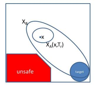
Figure 7: Safety region  $X_B$  vs. active safety margin  $X_A(x,T)$
