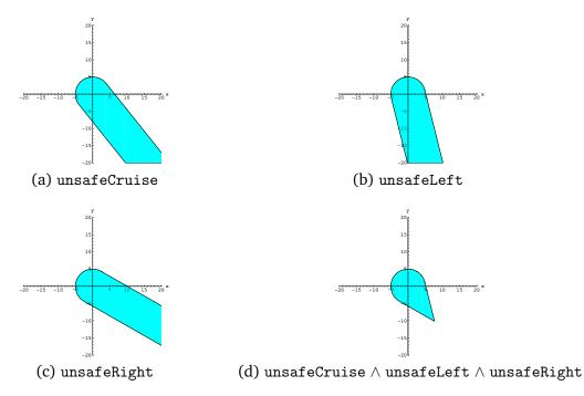
Figure 3: Showing minimal unsafe sets for each discrete state of maneuver automaton.
