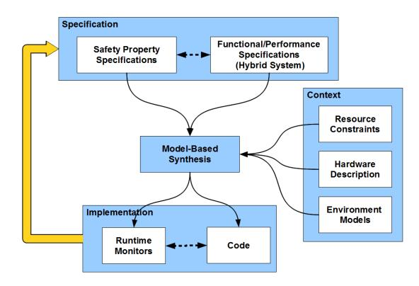
Figure 12: Model-based design flow for RTA.
