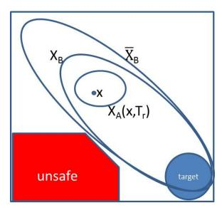
Figure 8: Enhanced safety region  $\overline{X}_B$  vs. active safety margin  $X_A(x,T)$
