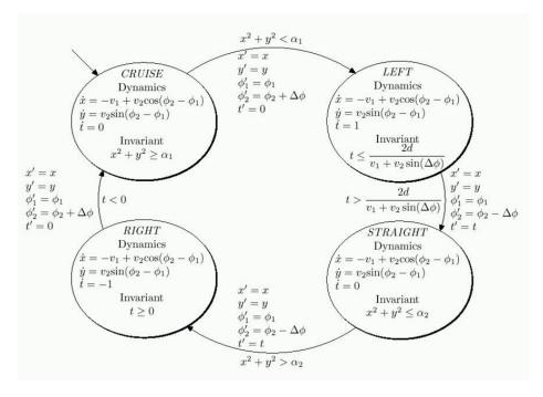
Figure 2: Hybrid system model of aircraft conflict resolution maneuver.
