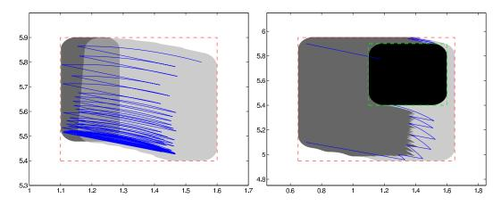
Figure 5: Example of switching safety (left) and reachability (right) controllers synthesized using approximately bisimilar discrete abstractions of a model of a DC-DC converter [41, 42].
