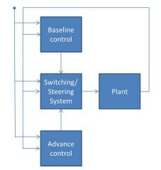
Figure 6: Run-time assurance architecture
